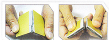
Low Quality Polyethylene core, will crack immediately after bending test.
