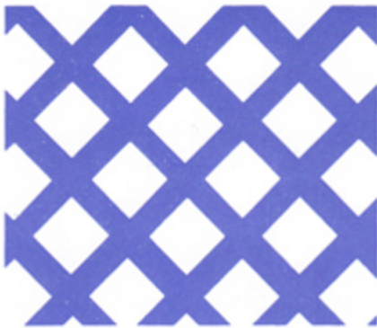
132 D7.5 x 11.5P 42.5% open .295" sq. diagonal, .452" centers
