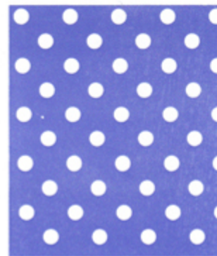
20 2.6 \phi x 9P .102" diameter .354" centers, 13% open
