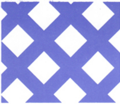
135 D10.5 x 17P 38% open .276" sq. diagonal, .669" centers
